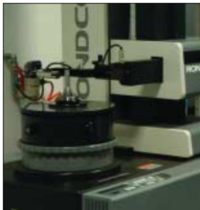
Rotor concentricity is measured to allow vibration-free operation.
